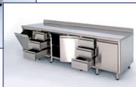
These neutral bases can be used to create equipped tables in AISI 304 scotch-brite satin stainless steel. The drawers have stainless steel guides with bearings, while the soaked container model has an internal support to hold the containers. It has hinged doors with adjustable internal hinges. In the standard version, all of the models are provided with adjustable legs that can be replaced with stainless steel wainscoting.
