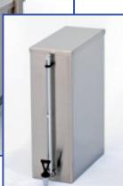
Our soaked containers are used in very busy pastry making workshops. They are fitted with a glass level sensor, a steam cock and a top lid. They have a capacity of approximately 25 litres. A set of guides can be fitted under the hanging cupboards, which can be used to house a certain number of small drawers. These are comprised of a 1/3 gastronom container with a handle on either one or two sides. All of these accessories are designed in AISI 304 scotch-brite satin stainless steel.
