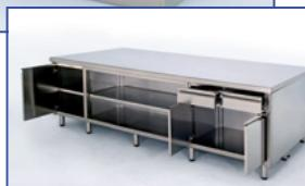
These neutral bases can be used to create equipped tables in AISI 304 scotch-brite satin stainless steel. All of the models are provided with a reinforced, adjustable middle shelf. Furthermore, the standard version has adjustable legs that can be replaced with stainless steel wainscoting. The doors can be either sliding doors on guides with ball bearings or hinged with internal adjustable hinges.
