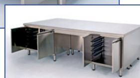
These neutral bases can be used to create equipped tables in AISI 304 scotch-brite satin stainless steel. The base is equipped with 6 double guides for pastry and bakery trays. The 1000 mm wide model has double internal guides. In the standard version, all of the models are provided with adjustable legs that can be replaced with stainless steel wainscoting.
