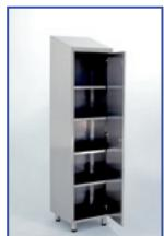
Designed in AISI 304 scotch-brite satin stainless steel with a welded, monobloc frame. The cupboards have double-panelled hinged door with adjustable, internal hinges are equipped with a lock and key. Available both in 500 mm version with a single door or in a 1000 mm version with a double door, containing shelves, a broom holder and a clothes rail. The 1000 m clothes rail has a central divider. All are provided with adjustable feet and a sloped roof of 18° for easy cleaning.
