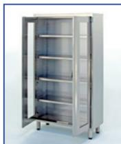
Designed in AISI 304 scotch-brite satin stainless steel with a welded, monobloc frame. The cupboards have double-panelled hinged door with adjustable, internal hinges are equipped with a lock and key. 3 middle shelves, 2 of which are adjustable, are also provided. The legs have an adjustable foot. We also offer a version with transparent doors. In this case, the inner shelves are available smooth, as well as drilled or in glass.
