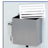
These units are used to sterilize knives and other implements and are offered in three different versions: neutral immersion, heated to 83 °C and with UV-A rays. The heated and UV-A versions are 220V, single-phase powered.
